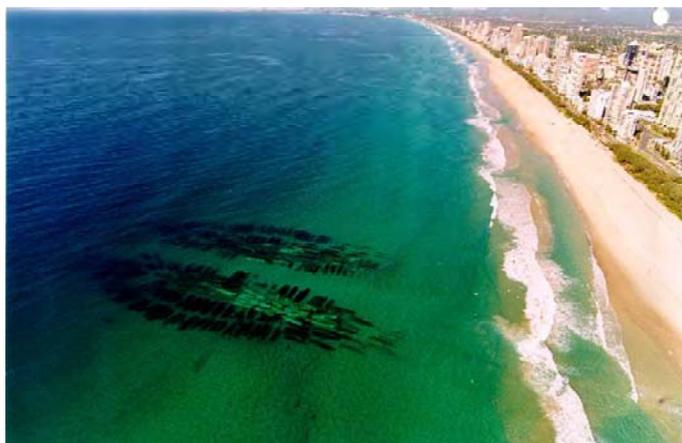
Fig. 1. Aerial view of the Artificial Surf Break at the Gold Coast, Australia. The structure is V-shaped in plan with the apex pointing seaward (courtesy of International Coastal Management, Australia, [www.coastalmanagement.com.au](http://www.coastalmanagement.com.au)).
